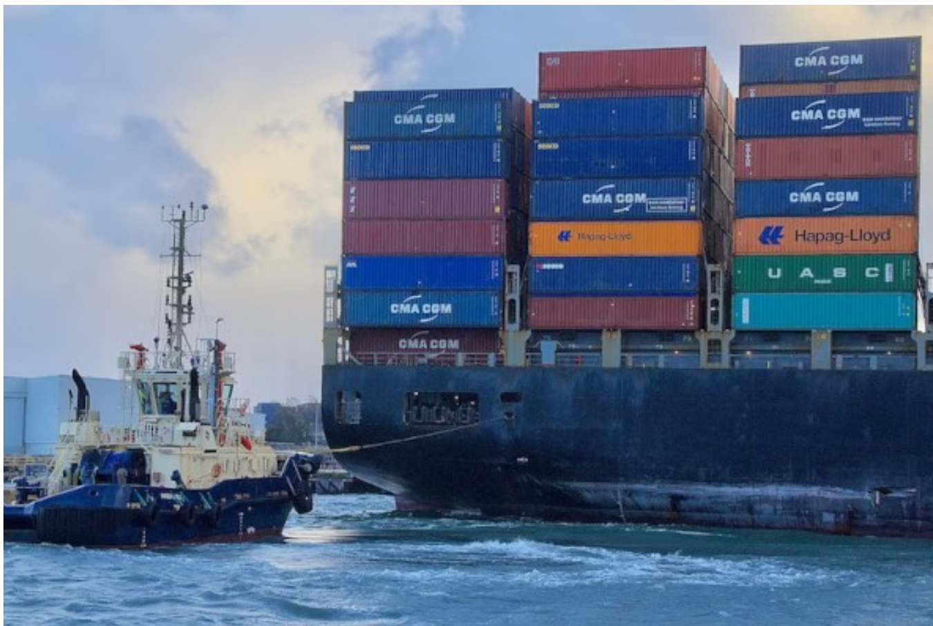
The ship following the collision of its stern and the wharf. The hole punched in the side and the scrape down the side plainly visible.
