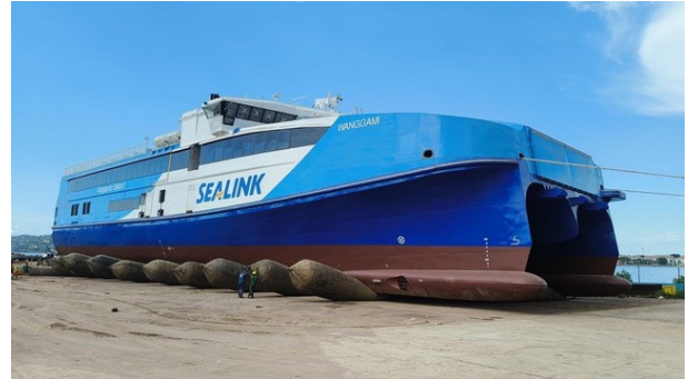
New SeaLink ferry Wanggami on rollers about to be launched at the shipyard in Batam, Indonesia, as published in October last year.
